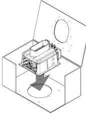
The Bowl Vent (4) and Bowl Lip (5) are fixed to the underside of the lid. In most cases this would be achieved using mechanical fasteners.
