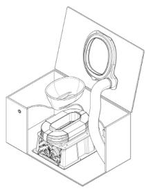
The Bowl (3) is simply placed onto the EFM. Opening the hinged lid gives access to remove the Bowl, which is necessary to install new Liners. Closing the hinged lid engages the Bowl Lip with the Bowl to prevent urine from escaping the system.
